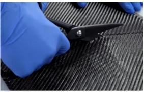
Figure 4: Cutting reinforcement of carbon fiber cloth
