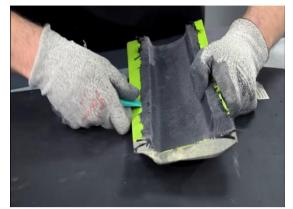
Figure 9: Demoulding of the cured part.
