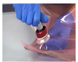
Figure 5: Preparation of the vacuum bag.
