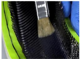
Figure 7: Lamination of the Part.
