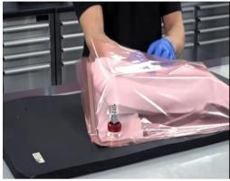
Figure 8: Vacuum bagging of the part.
