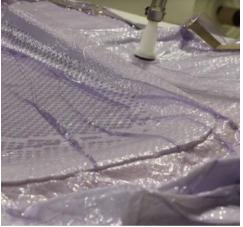
Figure 1: Vacuum Bagging Process
