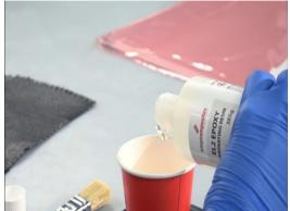
Figure 6: Measuring and mixing of the resin
