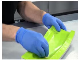
Figure 2: Application of mold release wax to the mold
